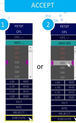
Press the EXECUTE button Click on the proposal, which makes the mouse cursor move automatically to EXECUTE and press EXECUTE
