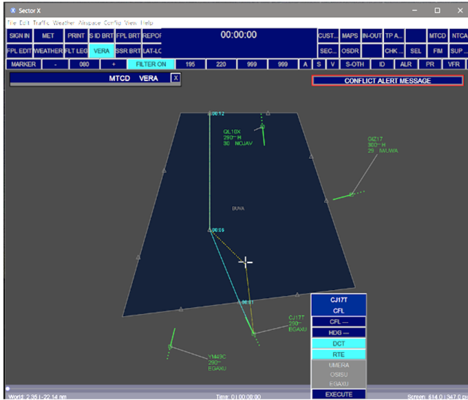
Figure 5. State of the art PVD implemented in SectorX
